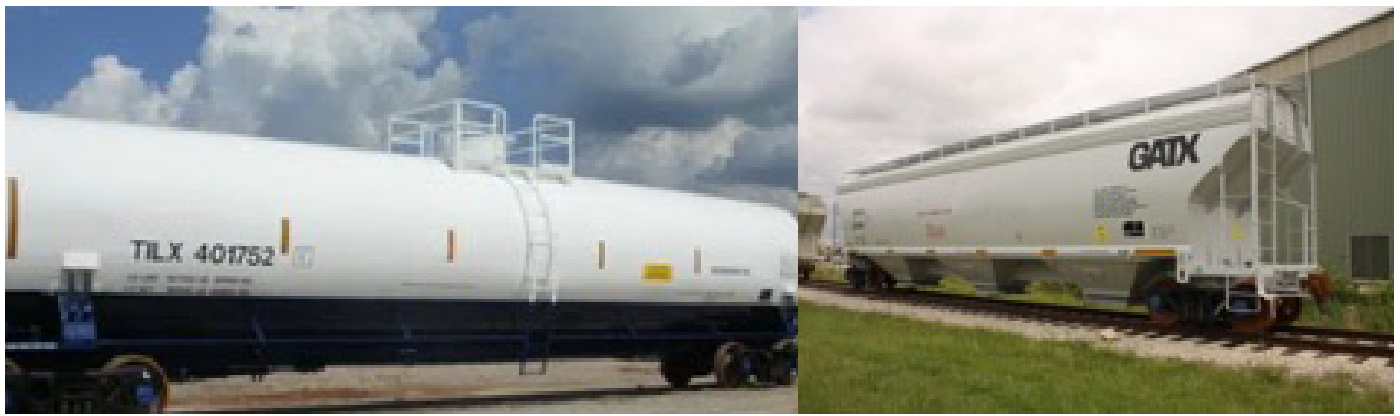
Figure 5-5. (left) The Trinity DOT 105 tank car for transporting liquid CO 2 and (right) a covered gravity hopper (> 5000 cubic feet) for transporting bulk-waste biomass.
