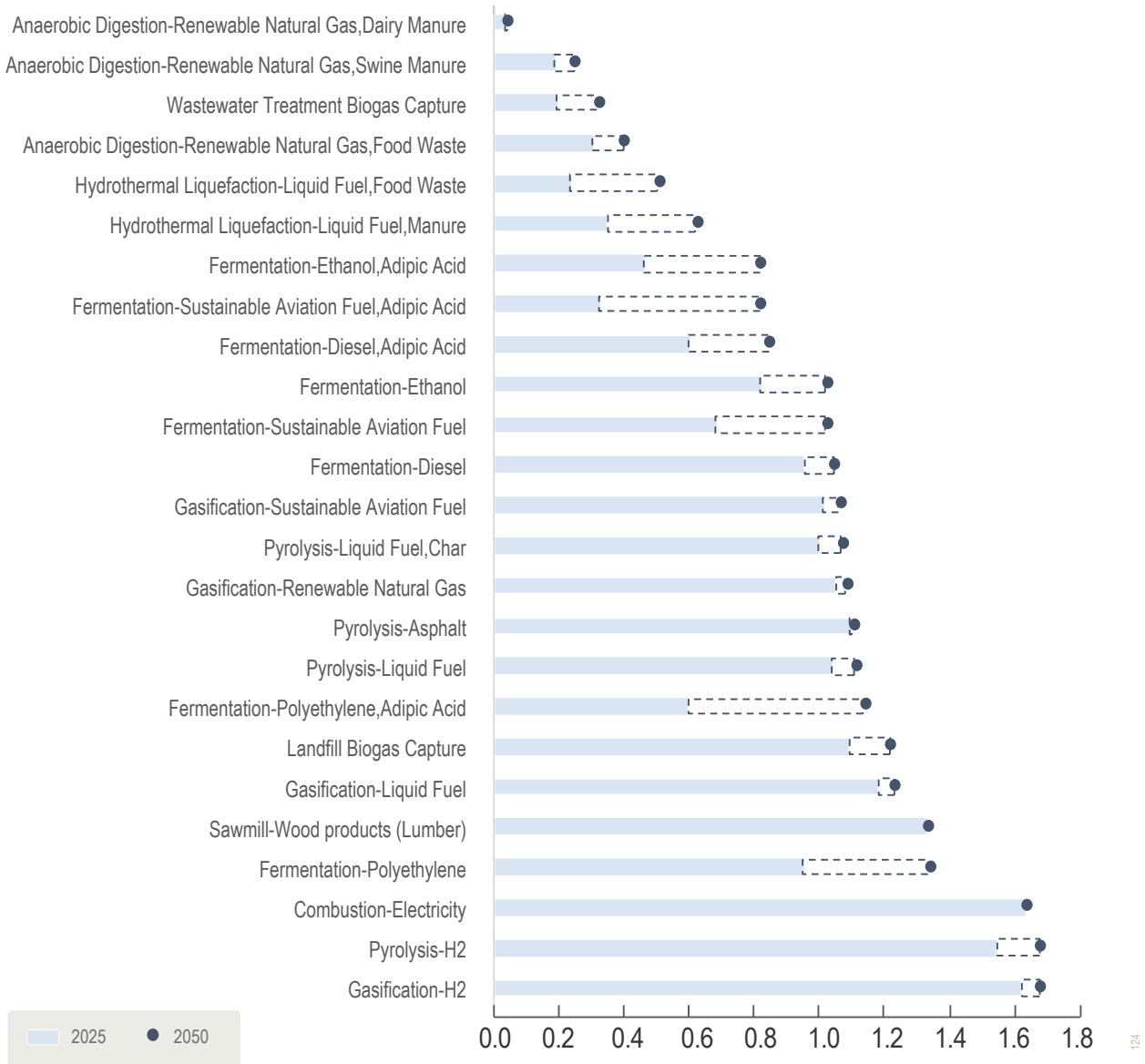
Figure 6-32. Projected 2025 and 2050 grid and hydrogen emissions impact on biomass CO 2 -removal potential on a “per dry tonne of biomass” basis. The analysis assumes a net-zero-emissions grid and net-zero-emissions hydrogen production for 2050, while utilizing current emissions factors for the grid and hydrogen production in 2025. The figure highlights findings based on a baseline biorefinery scale of 1000 dry tonnes of biomass per day. It specifically focuses on carbon removal at the biorefinery gate, excluding emissions associated with biomass harvest and transportation, CO 2 transportation, and injection.
